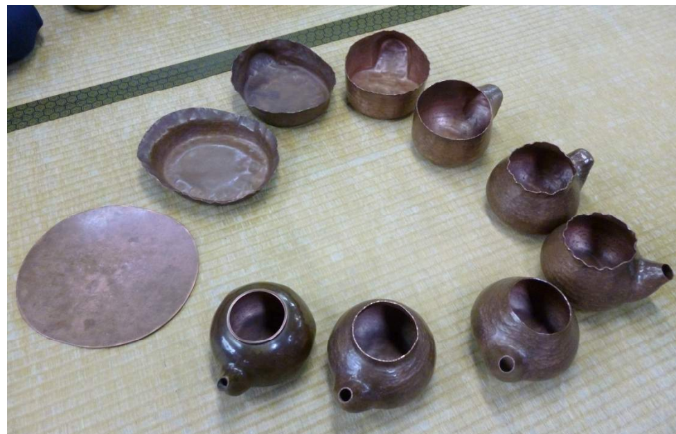
Stages in making a kettle by handraising (hammering and heating copper) at Gyokusendo
